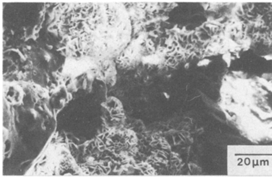
Figure 11 Debris at the surface of the GRP rod at the point of electrical breakdown. The small platelike crystals are very rich in zinc.
