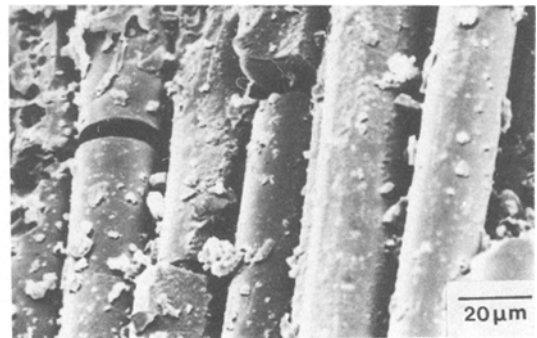
Figure 18 Higher magnification picture of transverse cracks in the surface regions of the rod shown in Fig. 16.
